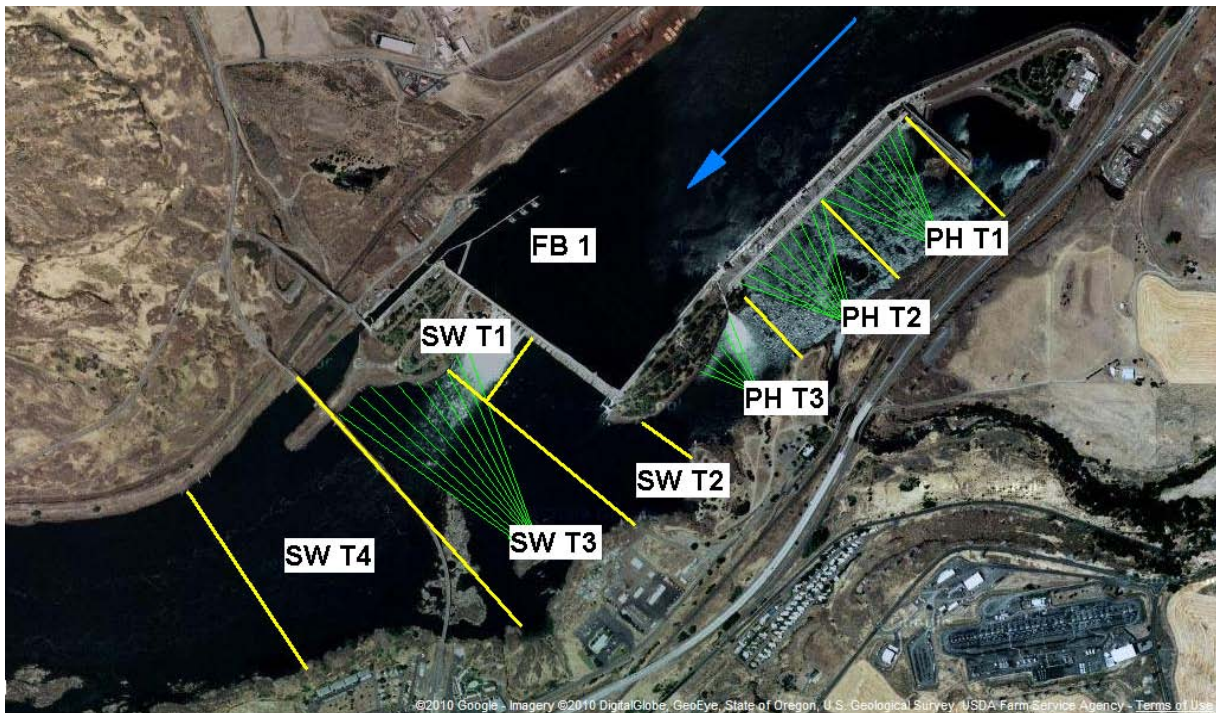
Figure 3. Image of The Dalles Dam at Columbia River mile 192 (©Google Images 2009). Flow is from right to left with the 2011 avian array represented by thin green lines and the observation zones demarcated by yellow lines.
